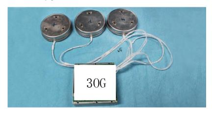
The 3OG consists of body and heads, there are lines between the head and the body, the lines' bending radius is demanded not less than 30mm. The gyros are recommended for using in an enclosed environment, and keep the gyros dried, otherwise, it will do damage to the precision and service life of gyros.
